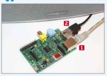
Connect your Pi to both an Ethernet network 1 and some speakers. 2 You don't need to connect a monitor, keyboard or mouse, because MusicBox is controlled through a web interface, but a monitor will help you find the Pi's IP address in Step 3. Before plugging the Pi into a power socket, you'll need to install the Pi MusicBox OS on the SD card.
